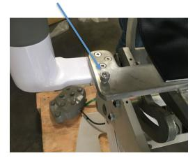
6. Align the seat cushion mounting holes with the seat frame. Secure the seat cushion to the seat frame using the 2 (5MM) Bag (E) Allen screws and washers.
