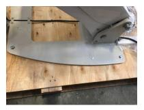
3. Remove the lift handles from the pallet. Install on the threaded hub on each side of the chair. These are going to be used as a lift point. Do-not use the chair armrest as lift points.
