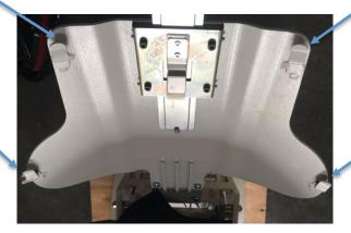
2. Once all 4 tabs are aligned with the backrest cushion slots, Slide the backrest down to secure in place. Verify all 4 corners are secured.
